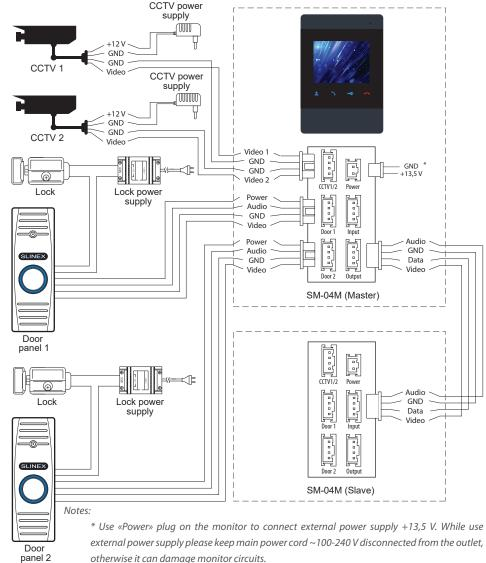
\*\* Door panels, cameras, power supplys and locks, described on the diagram are optional devices and are not included into monitor kit.
